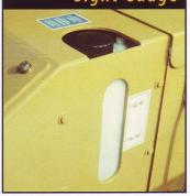
Radiator coolant level sight gauge = visual service checks.
