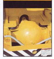
Meritor design axle = increased load capacity & mechanical differential lock.
