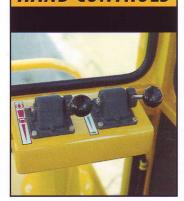
Rear brake/throttle hand controls = convenient operation from the rear operating position.
